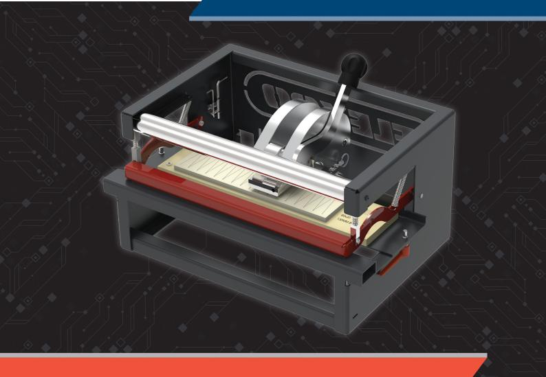
Novitool® Pun M™ Mobile Punch Prepare Finger or Finger-Over-Finger Splices
